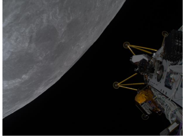
Figure 2: Photo taken by lander (same camera as Figure 1) in low lunar orbit featuring the PRIME-1 payload. Note that all mechanisms and faces are clean.
